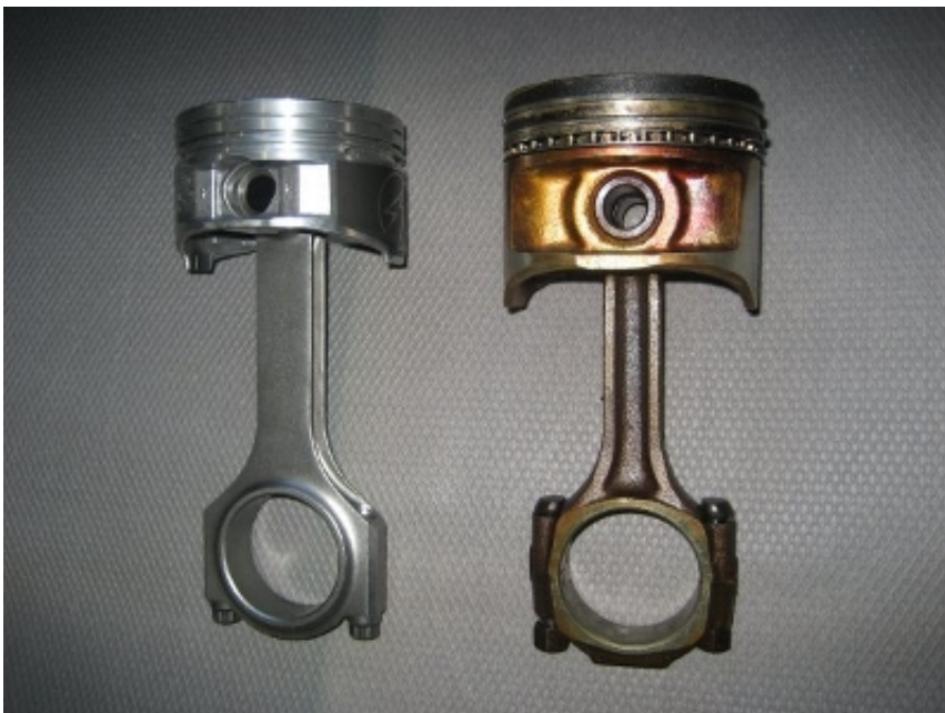
On the left is a 5.71" Olds Quad4 rod with a Cadillac Northstar
