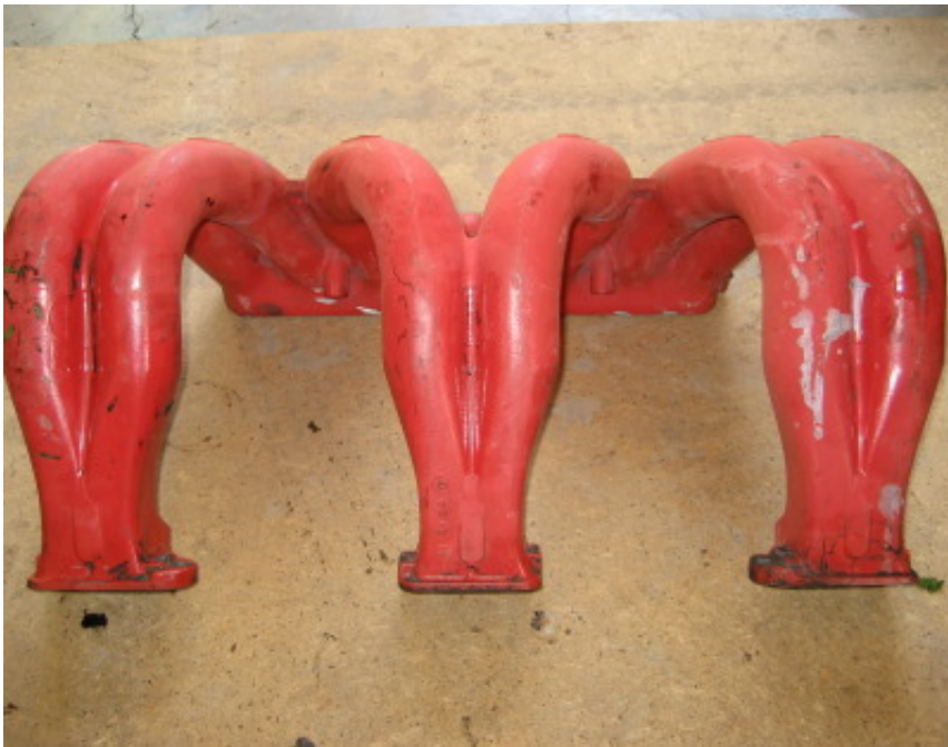
This shot shows how the manifold runners neck down as they approach the head.
