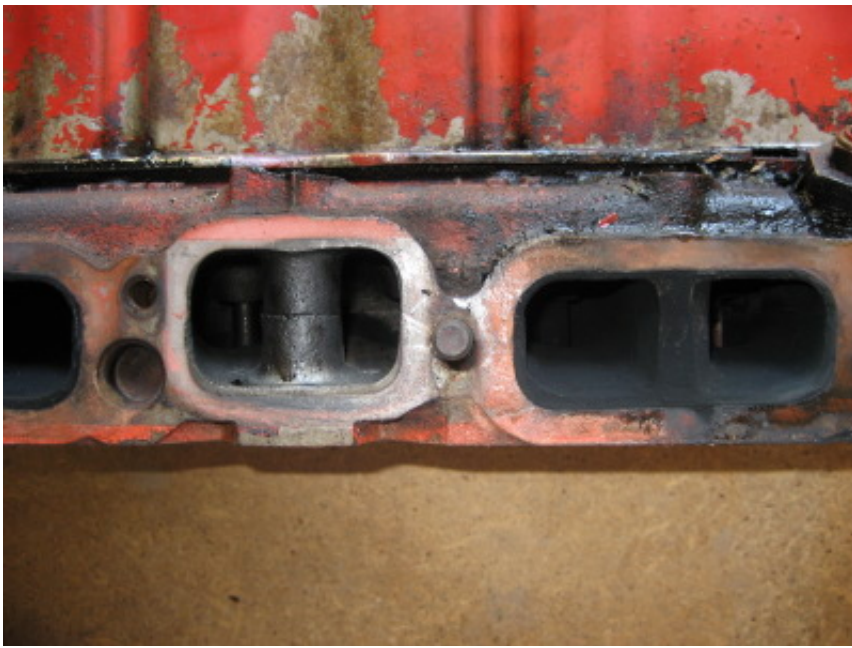
Nine port head from a red 202. Note the thick bolt boss in the intake port.
