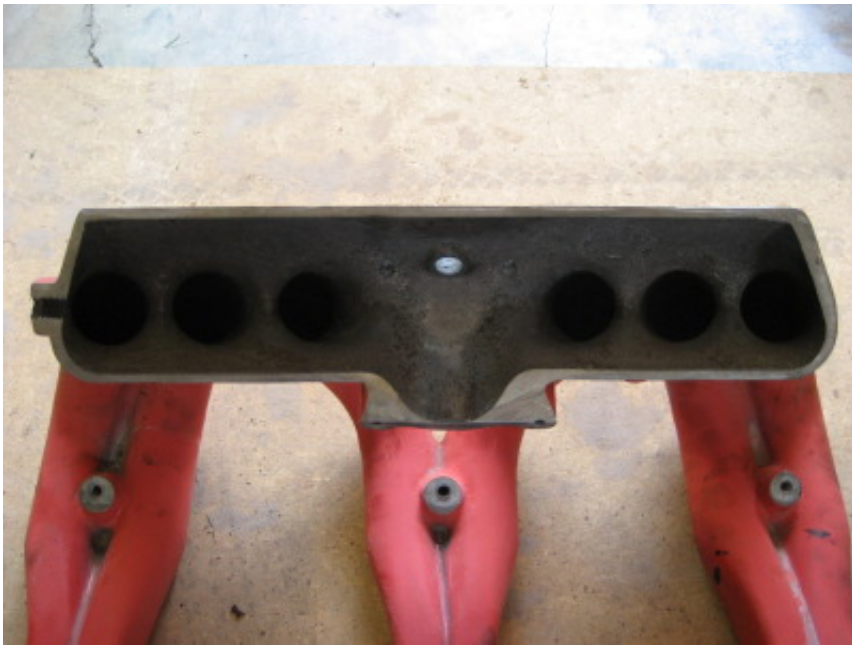
VK EFI manifold sectioned to show the 40mm ID runner entries.
